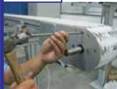
Stretch the chain and remove links if necessary so that the chain slacks slightly at the drive unit. Connect the chain ends.
