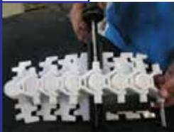
Align the chain tool with the pin. Slowly press the trigger until the pin is inserted.
