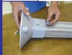
Slide the connecting strips or square nuts into the structural beam T-slots.
