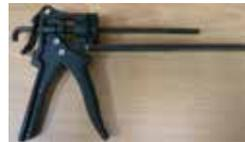
Chain pin insertion tool shown without attachment and specific drive pin
