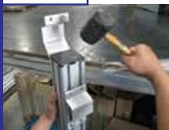
Use a soft hammer or mallet to clip end cap on to the support beam.
