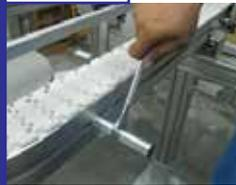
Tighten the distance tube to the set screw.
