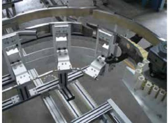
Automated side guide installed at bend section
