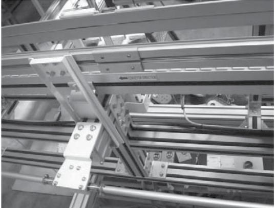
Automated side guide installed at straight section
