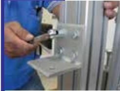
Mount the angle bracket to the beam in the same manner. Tighten all screws.
