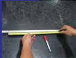
Mark the length of the rail to be bent. Leave an approximately 200mm straight section at each end.
