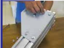
Mount the connecting plate to the beam using screws and washer.
