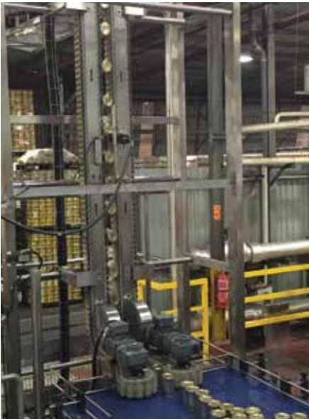
Stainless Steel Gripper for Tin Can Handling
