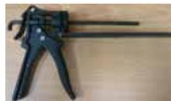
Chain pin insertion tool shown without attachment and drive pin
