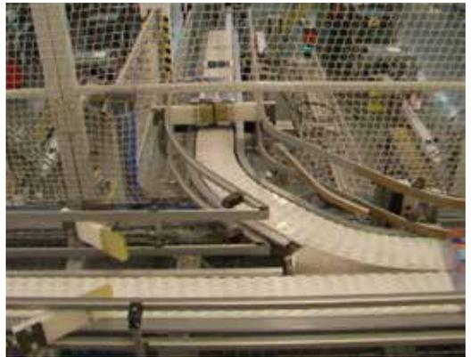
Pneumatic Traffic Controller for Merging
