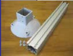
Insert hex head screws and washers into the holes on the side of the foot.
