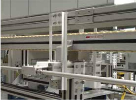
Automated side guide installed at straight section
