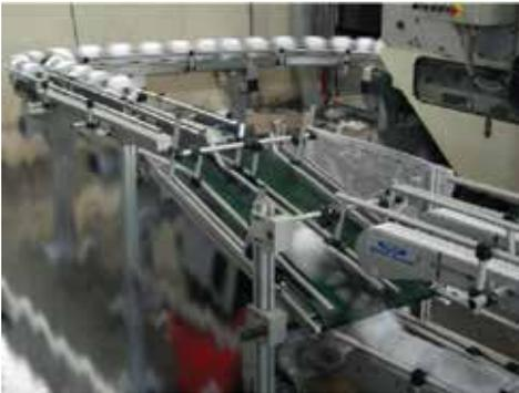
Vertical Diverter & Conveyor System for Tissue Rolls
