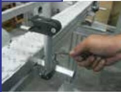
Attached the guide rail bracket to the distance tube. Tighten the screw.
