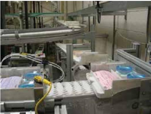
Side Transfer Unit for Optical Trays
