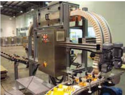
Gripper Conveyor System Intergrated with Can Cleaner to Remove Dust Particles from the Can
