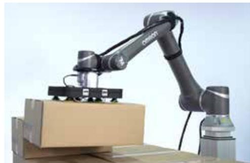
Cobot Palletizing using Omron Cobot
