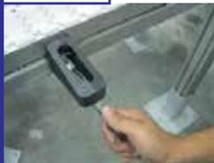
Insert square nut into T-slot of the beam. Fasten a guide rail bracket using hex head screw and washer.
