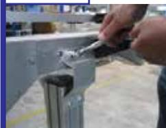
Mount the first support bracket to the conveyor beam. Bring the second bracket up and insert the T-bolts into the conveyor beam's T-slot. Tighten the nuts.
