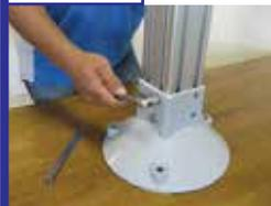
Tighten the screws using a wrench.
