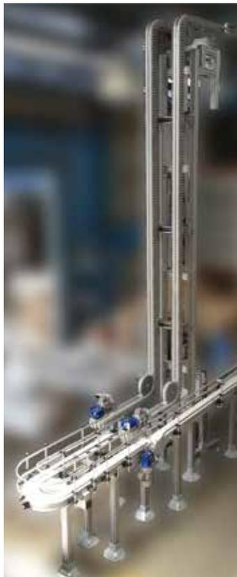
S-Flow Gripper Conveyor to Elevate Carton Boxes
