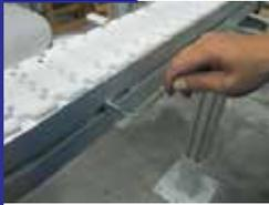
Insert square nut into T-slot of the beam. Insert set screw to the square nut.
