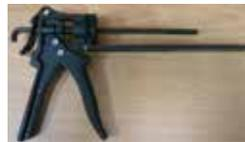
Chain pin insertion tool shown without attachment and drive pin
