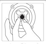
Rotate quill pin on speed reducer so that keyway is in 12 o'clock position.
