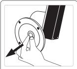
Remove plug from speed reducer.
