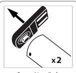
Remove drive pulley from bearings. (Take note of which side drive shaft is facing)
