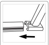
6 Slide secondary adjustment rod assembly into slots on guides.
