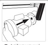
Install motor onto speed reducer.
