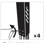
Looen but do not remove Looen but do not remove four cap screws holding bracket to frame legs.
