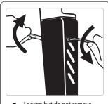
Loosen but do not remove safety bolt.
