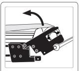
Using a box wrench rotate 3 Using a box where... disengaged position.
