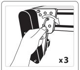
Tighten three cap screws on mounting package to conveyor.
