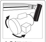
Rotate motor so 10 Rotate Illutur su workbox is in desired position.
