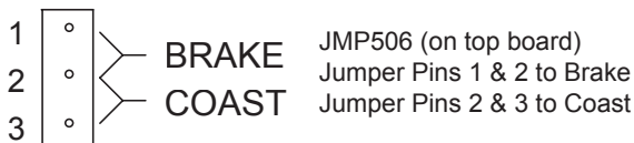
Figure 23. VFDP4X04 and VFD05 Jumper Settings--JMP506
